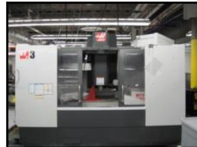
HAAS VF-3 Vertical Machining Center
