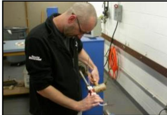
Rewinding Transformer for ASR-9
